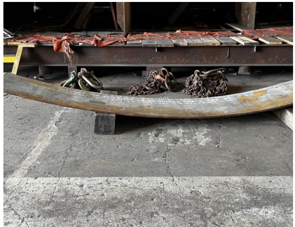
3143 – Guard plate after coming out of the break press. Conforms the plate to the curve of the vessel.
