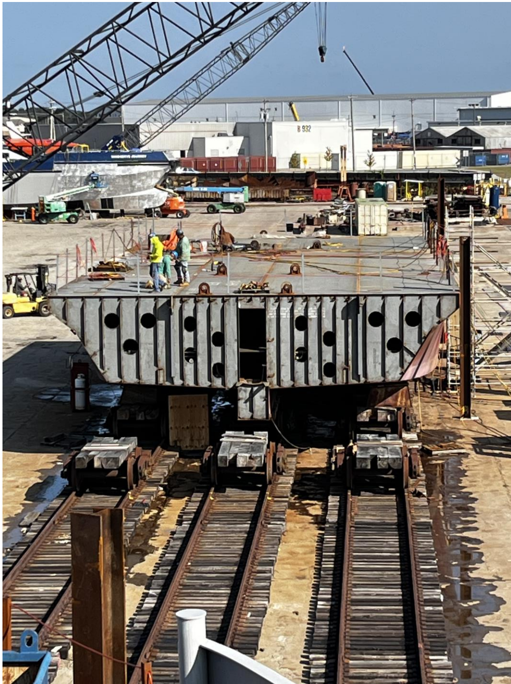
3264 – View of Portion of Shipyard and the first three modules being assembled. Working on deck welds.
