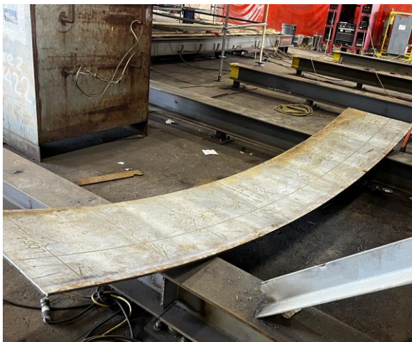
3146 - Guard plate after coming out of the break press. Conforms the plate to the curve of the vessel.
