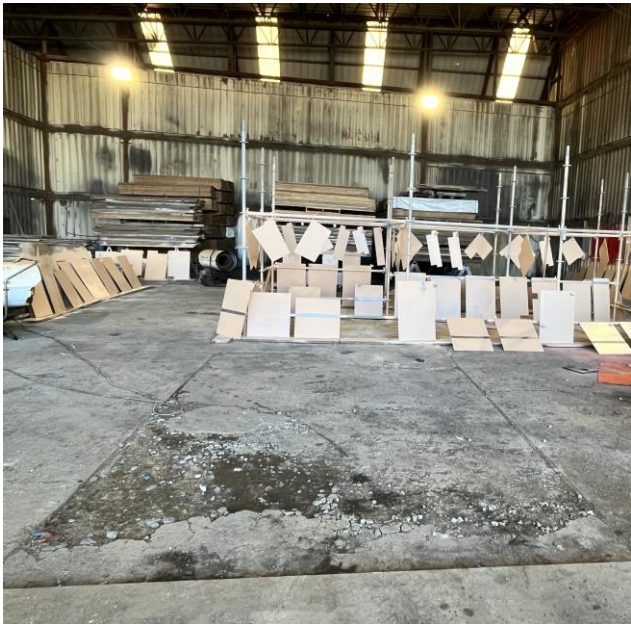
5752 – Floor Panel Sections Cut & Painted
