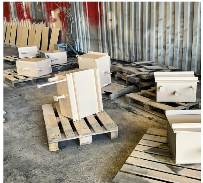
5753 – Cooling System Expansion Tanks Painted
