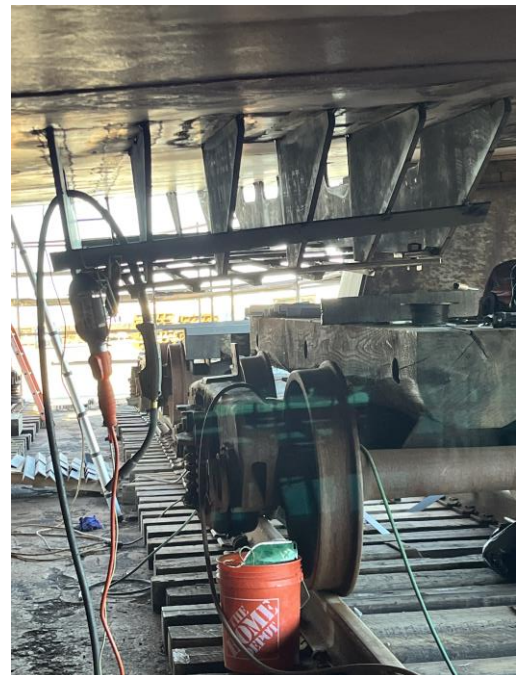
5576 - Installing Keel Cooler Guard
