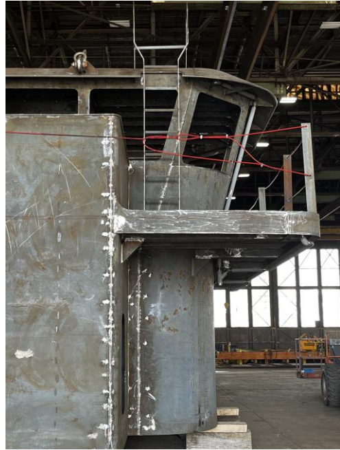
4353 – Pilot House w/Elevator Enclosure and Ladder Access to Mast/Roof
