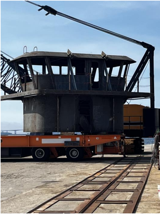
4422 – Pilot House Being Transported to Vessel
