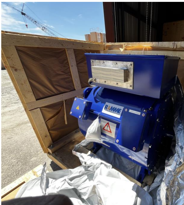
4417 – Electric Propulsion Motor
