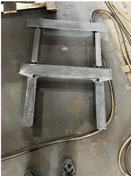
4310 – Framing Piece for Equipment Foundation
