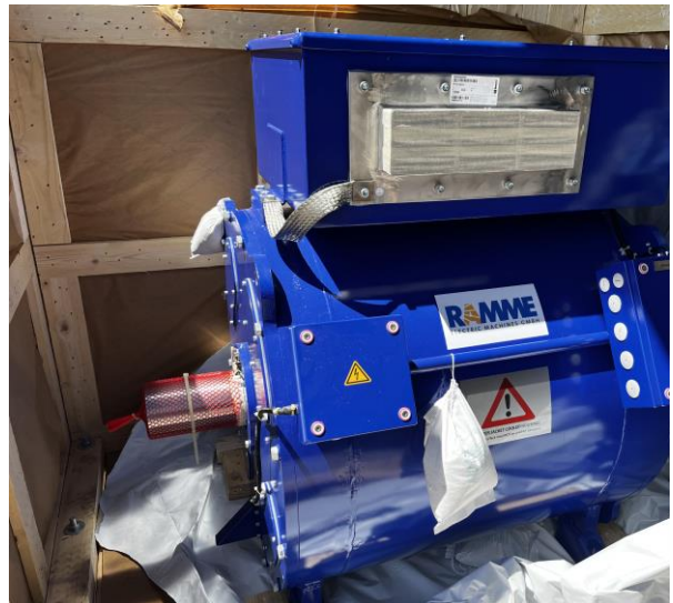
4415 – Electric Propulsion Motor
