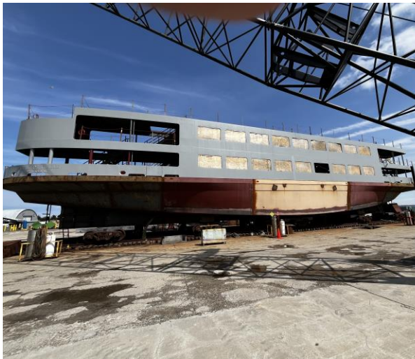
4377 – Super Structure Starboard Side – Next Paint Coat
