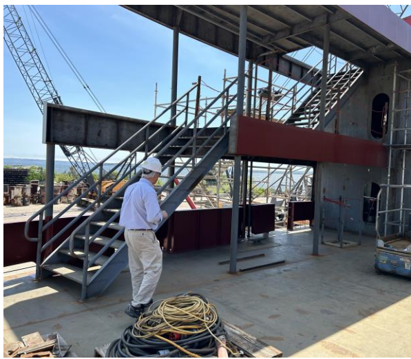
2522 – Starboard Bow Stairs and Cabin Openings (doorways are not cut in yet)
