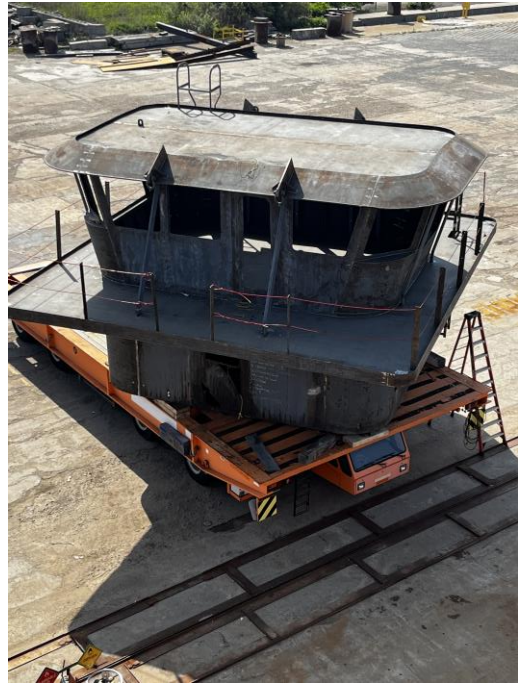
4426 – Pilot House in Place for Lifting
