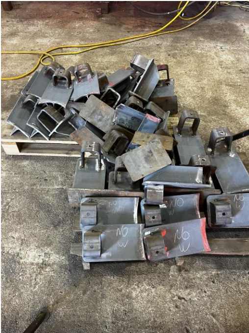
4387 – Exhaust Piping Brackets for Support
