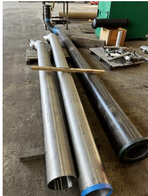
4383 – Exhaust Piping Both SS and Cast Iron
