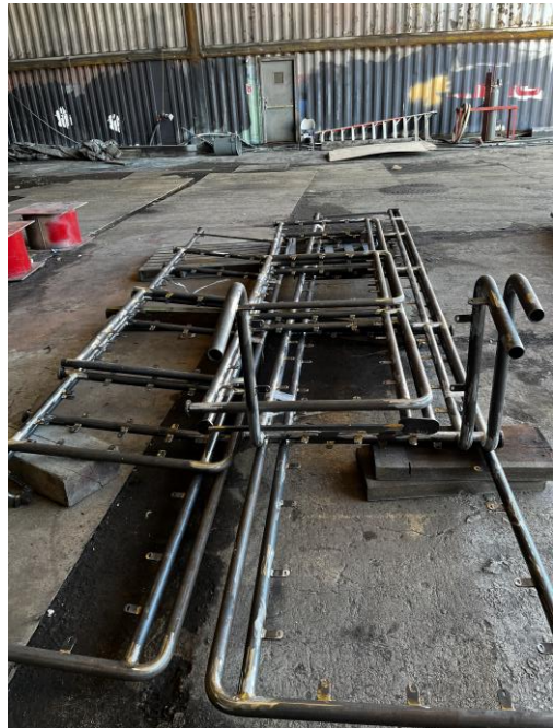
4578 – Handrail Sections Fabricated
