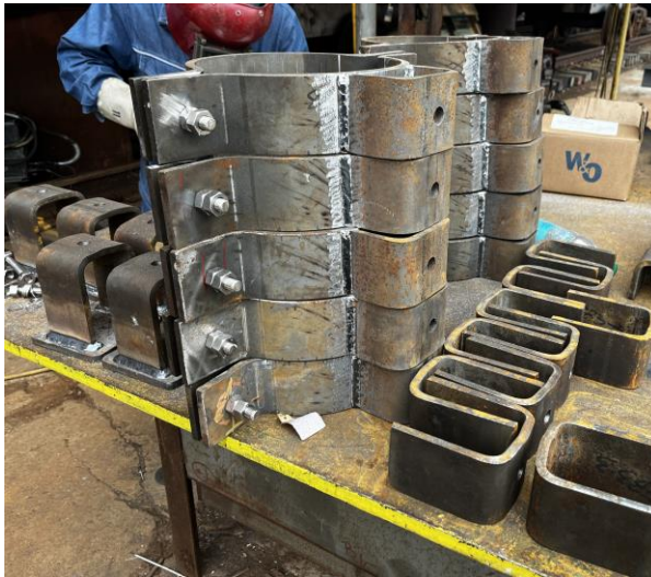
4762 – Piping Clamps & Supports
