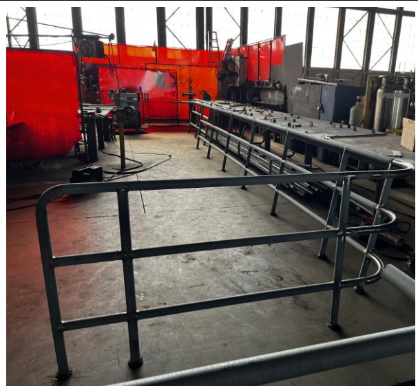
4620 – Handrail Sections Assembled and Primed
